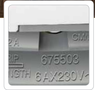
Laser marking safeguards against fakes
